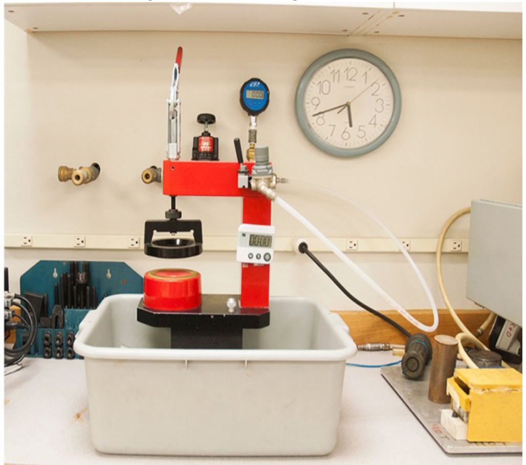
A fabric's waterproof rating is measured in mm, which represents the pressure at which water is able to press through the fabric. Photo: MSR Summit Register
