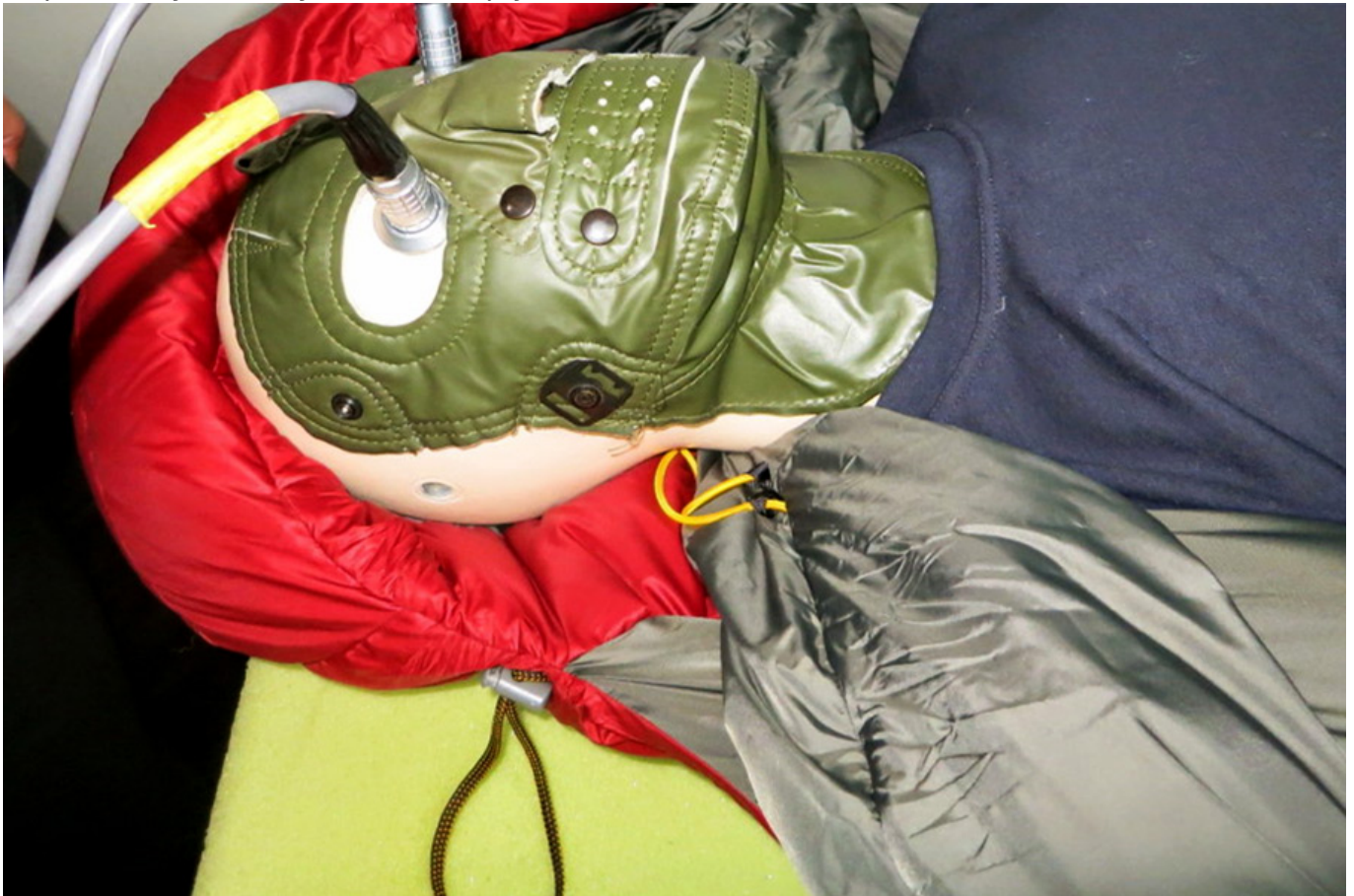
Here's the scary looking manikin during the EN test. Image: Sea to Summit.
