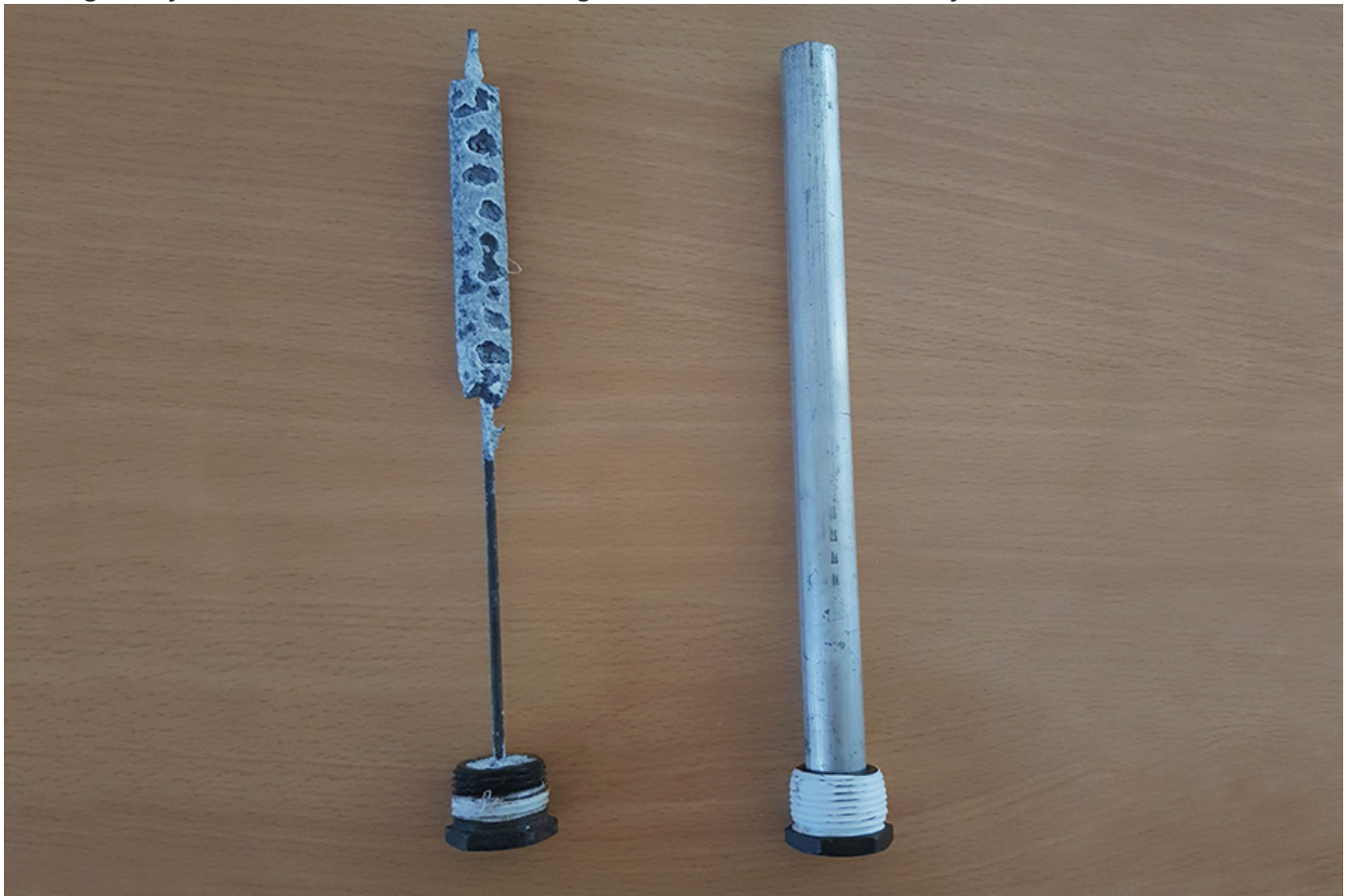
Pictured left: a used sacrificial anode, half corroded away
