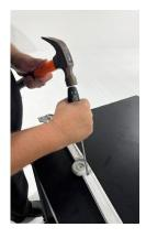
The replacement Hinge can be inserted into the extrusion and gently tapped into place using a rubber hammer or similar.
