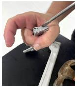
If it is desired to preserve the hinge fitting, it can be 'tapped out' using a screw driver/ chisel and a hammer. Note that you will need to fully secure the frame in bench vice or similar.
