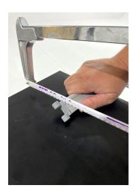
Alternatively, the Foot Fitting can be 'tapped out' using a screw driver/chisel and a hammer. Note that you will need to fully secure the frame in bench vice or similar.
