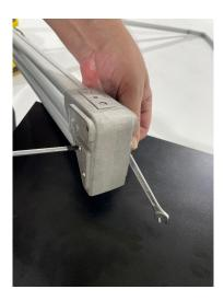
It will be necessary to remove the Foot Fitting from the end of the frame segment. This can be achieved by either cutting off or 'tapping out' the Foot Fitting as described above.
