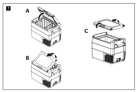
The lid can be opened from either side or removed completely without the need of tools as follows:
