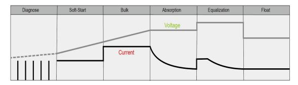
**Diagnose** \* – Only for Lithium battery type, subjected to the Lithium battery initial voltage then determine if going to Soft start or Bulk charge; if the Lithium battery is protected by BMS, the controller will automatically send the signal periodically to the battery terminals to activate the BMS against protection.
