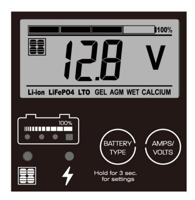
Press **BATTERY TYPE button** and hold for 3 seconds to go into your battery type selection mode, the battery type you select will be shown on the LCD meter, the default setting is AGM Battery; the controller will automatically memorize your battery type setting.
