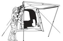
Throw the fly over the Tent and secure all plastic clips at the bottom. Secure Velcro straps after fitting.
