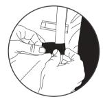
Fix the panels to the awning poles with the attached Velcro straps.
