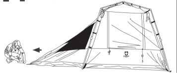
Assemble the Extension Pole. Feed the Extension Pole gently through the sleeve at the back of the Tent. Allow the pole to rotate freely for an easier feed.
