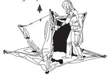
Pull all the arms out from the knuckles to lock the frame into place. You may need to push the Tent up a little to lock in the last knuckle.
