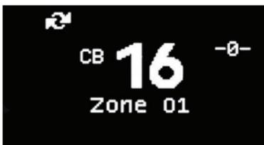
The radio returns to the main screen with the selected zone displayed below the channel number.
