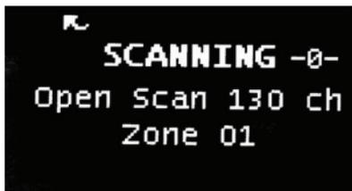
If there are less than 2 channels programmed into the scan memory when you press **SCAN**, a low beep will be heard and the command will be ignored.
