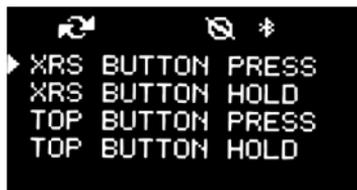
4. The XRS Button option list is displayed. The currently selected option is marked with a dot. Use the **▲** or **▼** keys to select to desired option then press **MENU** to select.
